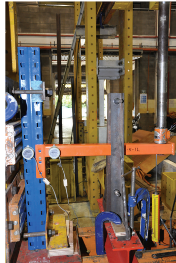
FIGURE 1: Typical flexural test for storage rack connection.
