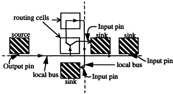
FIGURE 5 A route segment of a signal illustrating the sense of direction.
