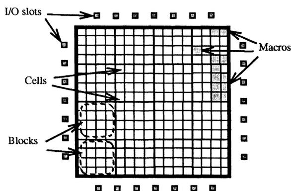
FIGURE 1 A simplified schematic of the FPGA architecture, where  $m = 4$ .
