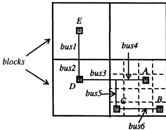
FIGURE 10 Inter-block and intra-block bus utilization.
