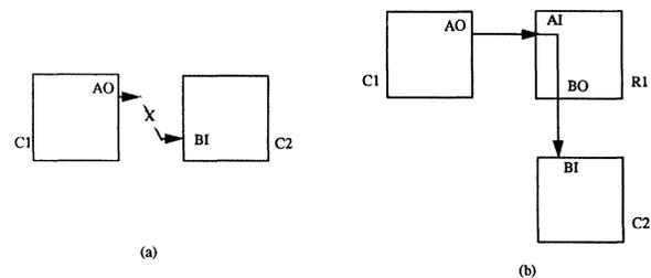
FIGURE 6 The scheme to get from pin AO of C1 to pin BI of cell C2.
