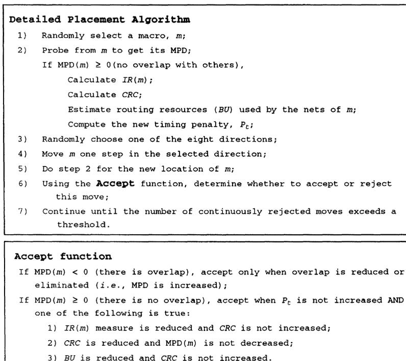
FIGURE 11 Detailed placement algorithm.
