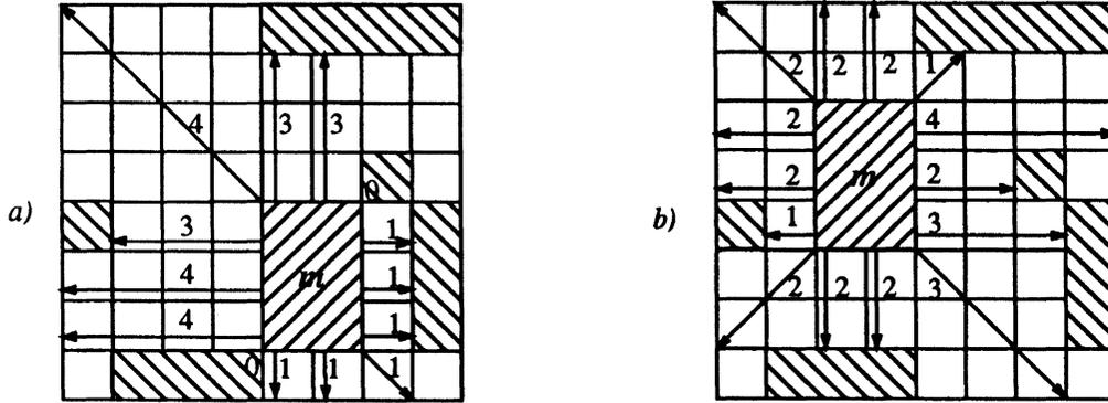
FIGURE 9.2 a) Probe distances for macro *m* after a one-step move in the SE direction. b) Probe distances for macro *m* after a one-step move in the NW direction.
