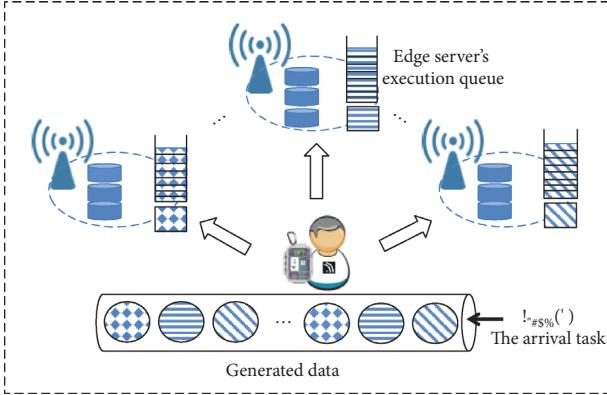
FIGURE 2: Computation task offloading framework with multiple edge servers.
