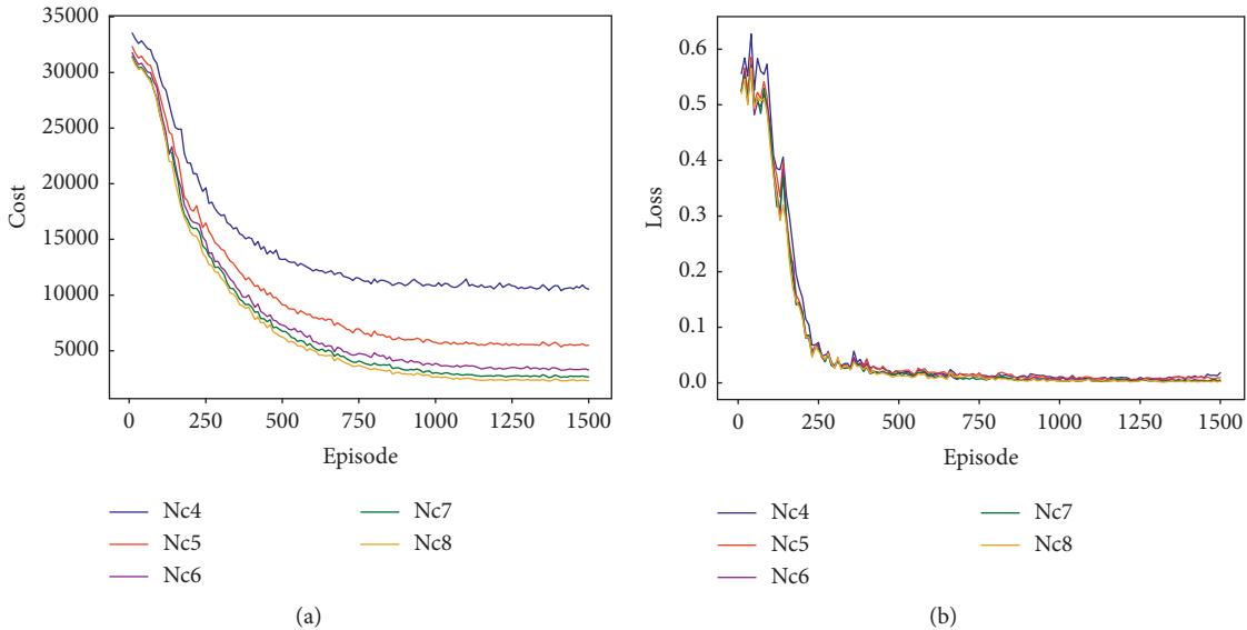
FIGURE 12: Learning curves w.r.t. different number of CPU cores.
