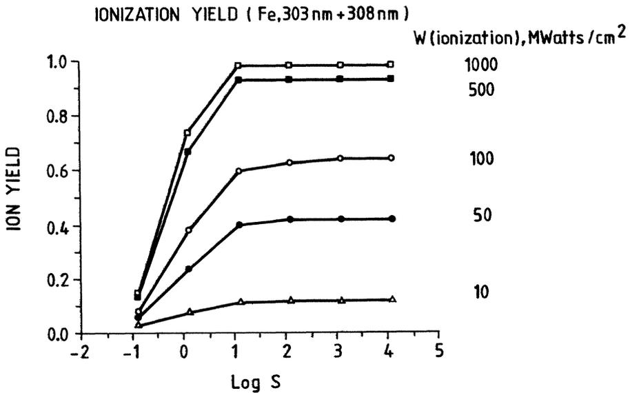
**Figure 1** Calculated ionization yield of Fe atoms as a function of probe and ionizing laser powers at the end of a 20 nanoseconds pulse.  $U_{\text{Saturation}} = 70 \text{ KWatts/cm}^2 \times \text{nm}$ .
