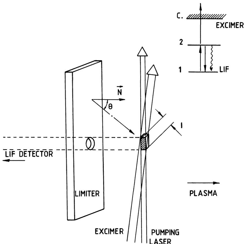
**Figure 2** Geometry assumed in the model calculation for a Be limiter. The interaction with the plasma is assumed to take place within a rectangle of 2 cm wide and 4 cm high. See text for the rest of the parameters used.
