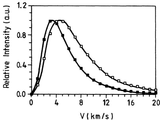
**Figure 3** Results from the model calculation: (a) Time evolution of the LIF signal. Thompson model for  $E_b$  (Be) = 3.32 eV (top) and  $E_b = 1.66$  (middle) and thermal distribution (bottom) for  $T = 2000$  K. (b) Velocity distribution along the detection line of sight for the  $E_b = 3.32$  and  $E_b = 1.66$  eV cases for the same geometry as above.
