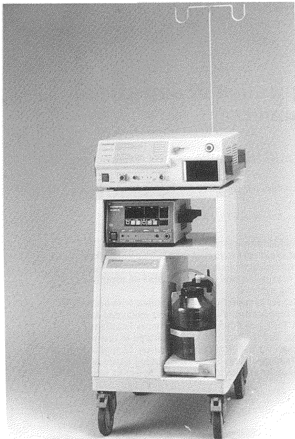
Figure 1 The generator of the endoscopic ultrasonic aspiration system (external dimensions 480 × 660 × 1070 mm) equipped with coagulation system (Surgical unit UES-10®).
