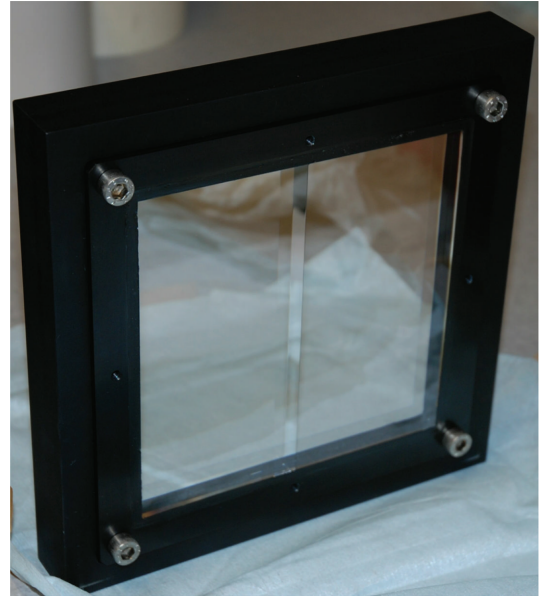
FIGURE 9: Photograph of a prototype of monolithic BGO assembly; it is made of two 20-mm-thick blocks and is 165 mm \times 165 mm in size.
