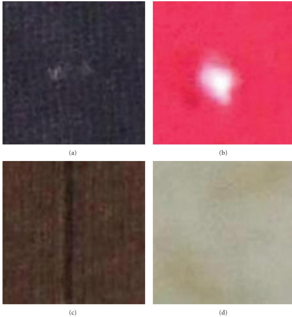
FIGURE 3: Different types of defects that occurred in knitted fabrics. (a) Color yarn. (b) Hole. (c) Missing yarn. (d) Spot.
