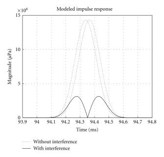
FIGURE 12: Overlapping Echoes associated with the Direct Path and the first Sea Surface Bounce.
