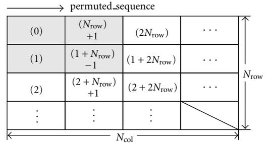
FIGURE 3: Permuted sequence from (1)–(2) for 16QAM.
