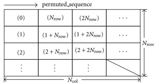
FIGURE 2: Permuted sequence from (1)–(2) for BPSK and QPSK.
