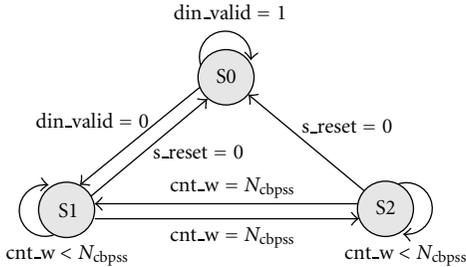
FIGURE 9: State diagram for the control FSM.
