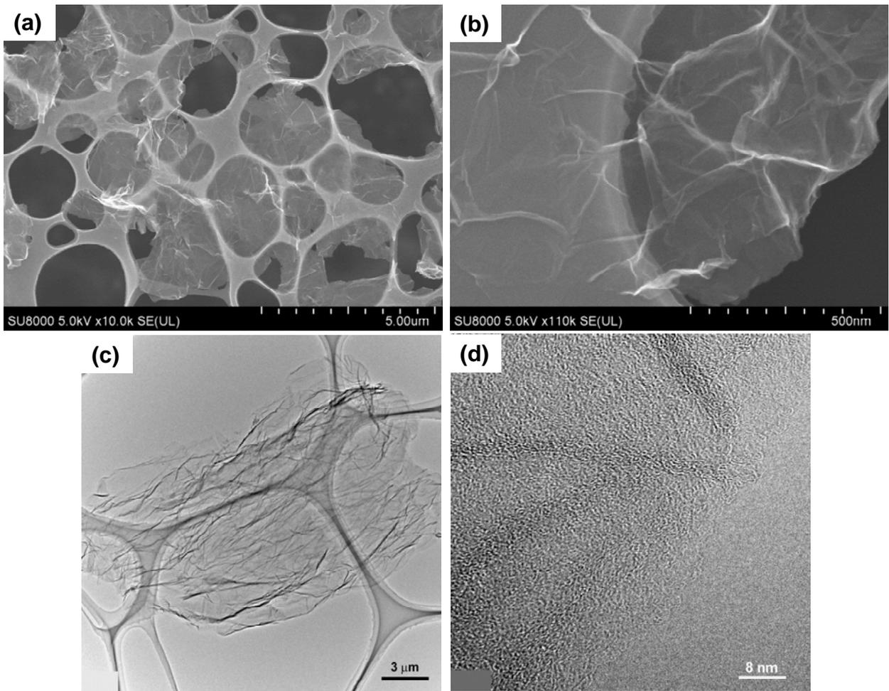
**Figure S-2:** (a) SEM and (c) TEM images of RGO sheets. High-resolution (b) SEM and (d) TEM images of individual RGO sheets. The sheets exhibit a crumpled structure.
