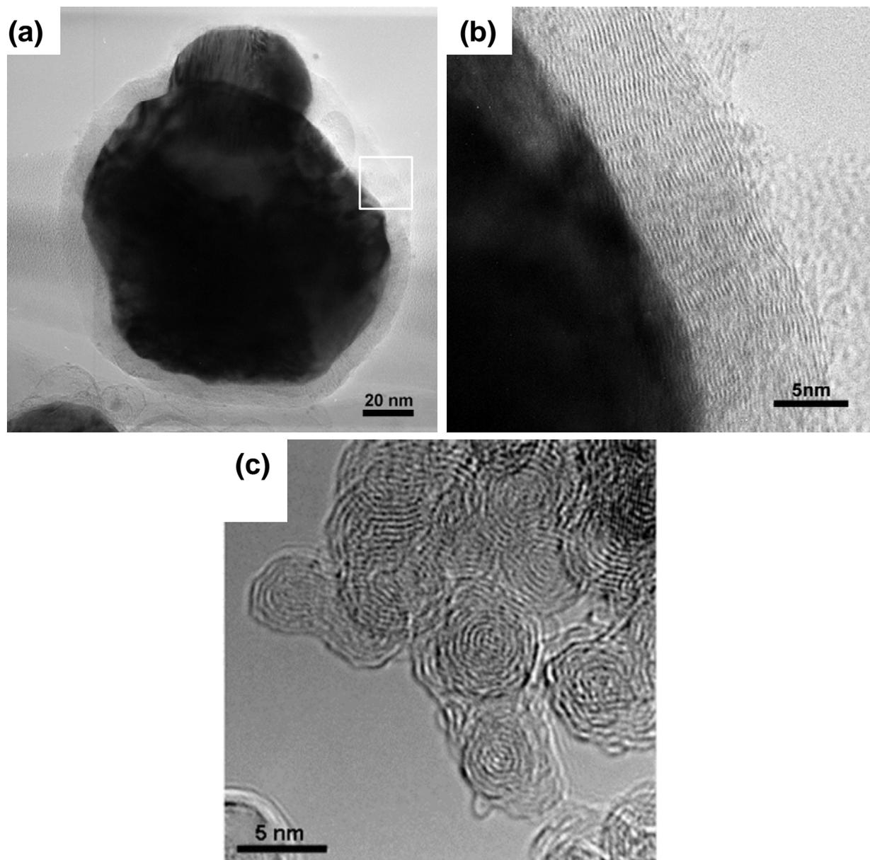
**Figure S-3:** (a) TEM image of a FePt@CNC. HR-TEM images of (b) graphene layers in the FePt@CNC shell marked in (a), and (c) carbon onions (Mykhaylyk et al. 2005).
