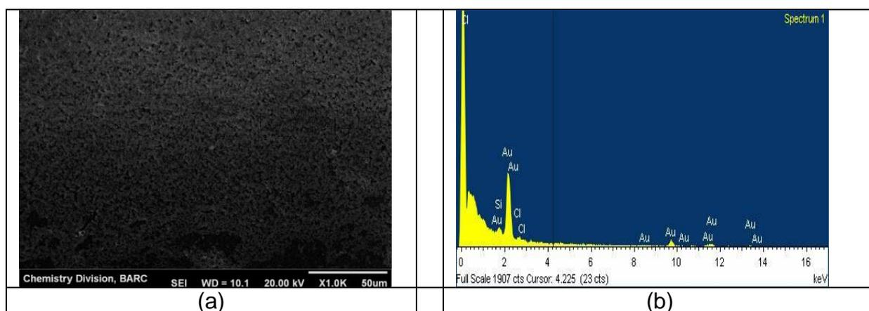
Figure S1: Scanning electron microscope image (a) and energy dispersive X-ray spectroscopy (b) of gold nanoparticles in 1mM SDS solution formed by the reaction of 1 mM  $\text{HAuCl}_4$  with 1 mM Trp.
