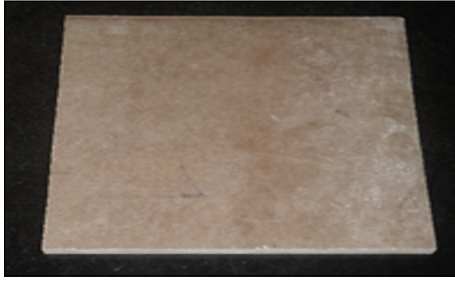
FIGURE 2: GFRP composite laminate fabricated by Hand lay-up process.
