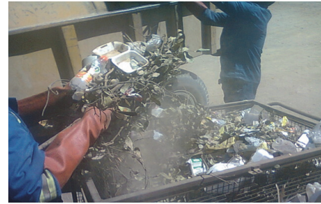
FIGURE 1: Dust generation from loading mixed waste without proper containment bags.
