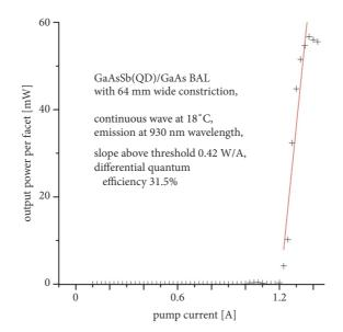
FIGURE 3: Laser characteristics of a confocal BAL with 64  $\mu$ m wide constriction just to show that the lasers are of very good quality. The laser threshold is at 1.2 A, and the output power per facet shows values around 60 mW for a pump current of about 16% above threshold.
