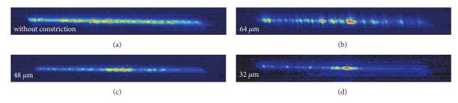
FIGURE 5: False-color plots of the near-field transverse intensity distributions for confocal BALs of the same batch with different widths of the constriction in the middle plane (i.e., no constriction, 64, 48, and 32  $\mu$ m wide, respectively). In all cases, the pump current has been around 16% above laser threshold and the lasers have been operated around 90 K in continuous-wave emission.
