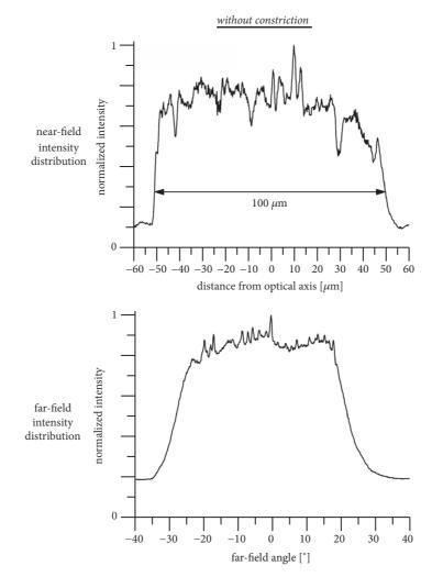
FIGURE 4: Near- and far-field intensity distributions for the confocal BAL without constriction, for comparison. The laser has been operated around 90 K in continuous-wave emission.
