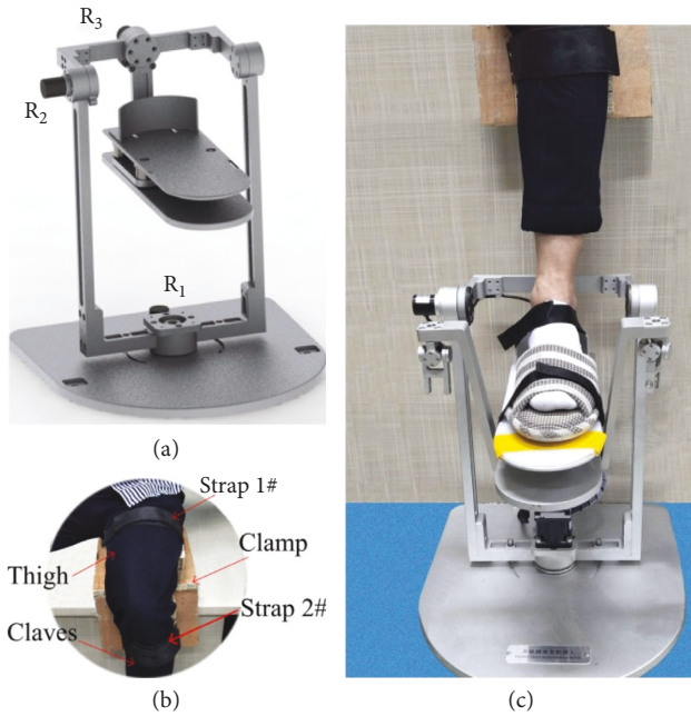
FIGURE 7: Measurement experiments of PMS. (a) RRR branch of PARR. (b) Wooden clamp. (c) Experimental platform.
