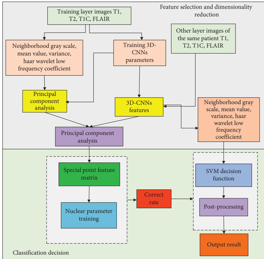
FIGURE 3: 3D-CNNs feature extraction method of MRI brain tumor subspace clustering algorithm.
