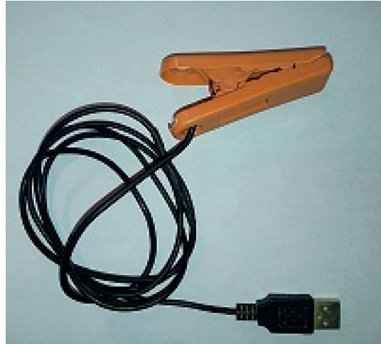
FIGURE 10: Finger probe used to fit the fingertip on the MAX30102 sensor. The sensor is placed inside the plastic holder.
