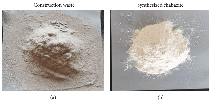
FIGURE 1: Pictures of (a) construction waste and (b) synthesized chabazite.
