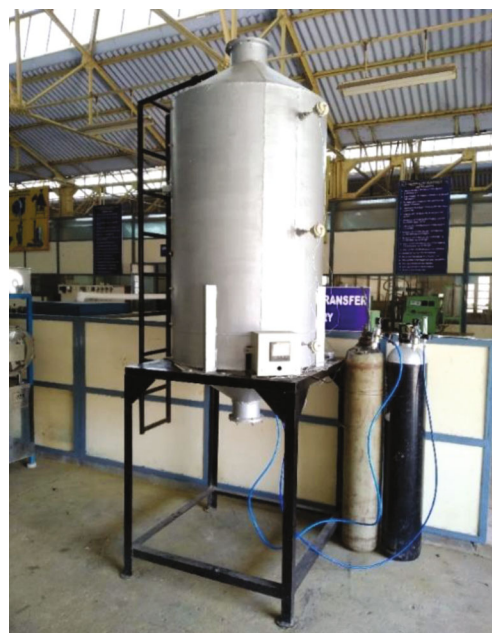
FIGURE 3: Experimental setup of controlled atmosphere storage bin for black gram grains.
