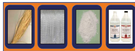
FIGURE 1: Photographic view of reinforcement/filler/matrix materials used in the current research.
