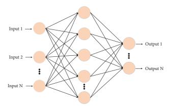
FIGURE 5: Standard connection methods for fully connected layer.
