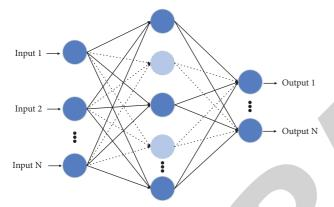
FIGURE 6: Fully connected layer with dropout connection method.
