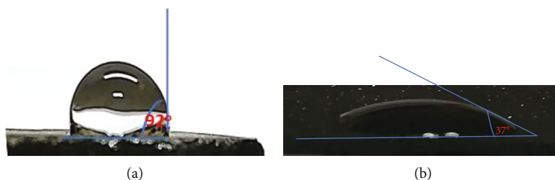
FIGURE 9: Contact angle values for (a) PANI and (b) PANI/Ag 2 O/Ag composite II.
