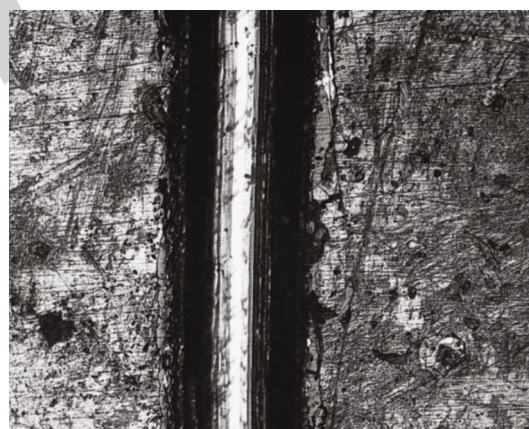
FIGURE 6: Wear track on DLC coating deposited on Al substrate.
