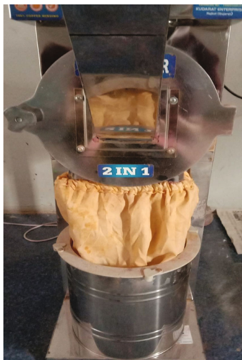
FIGURE 2: Showing the mini pulveriser machine, where the powdered flowers are collected in the stainless-steel collecting drum placed at the bottom.
