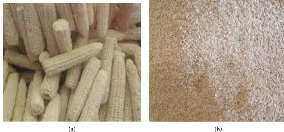
FIGURE 1: Raw corn cob samples: (a) before crushing and grinding and (b) after grinding.
