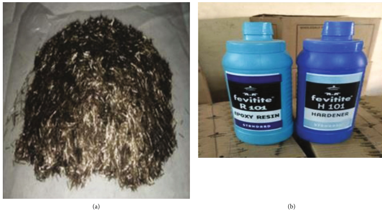
FIGURE 1: Main constitutions of epoxy composite (a) basalt fiber and (b) epoxy resin with hardener.
