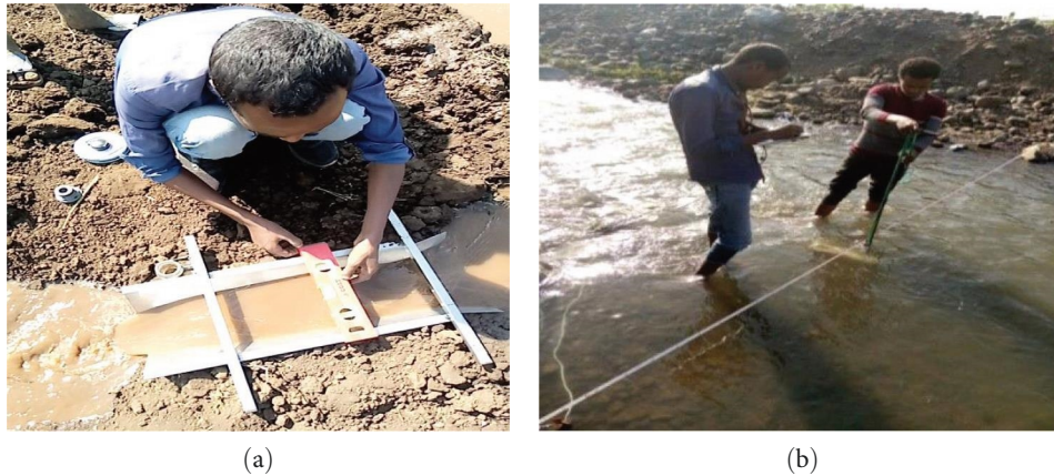
FIGURE 4: Measurement of flow at: (a) the farm inlet and (b) along the canal.
