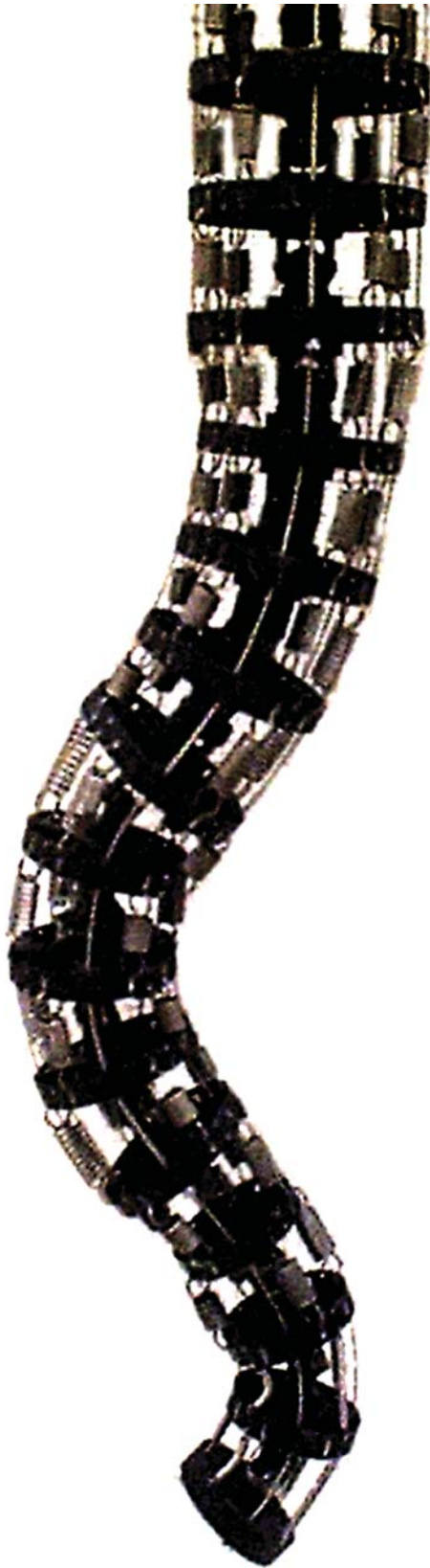
Figure 7. Elephant trunk manipulator, an example of hard hyper-redundant robot.
