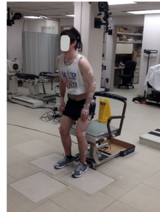
FIGURE 5: Data collection setup for the sit-to-stand and stand-to-sit trials.
