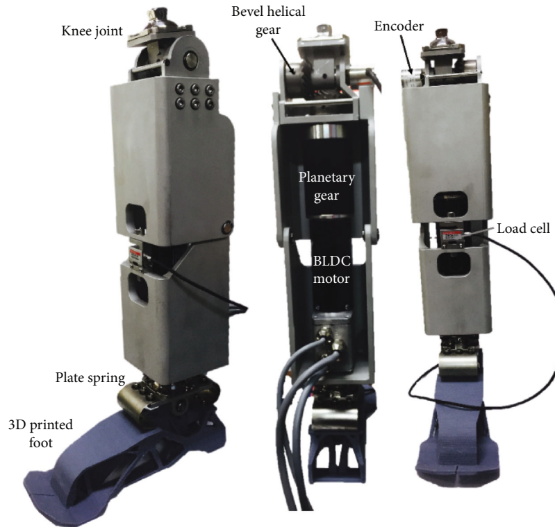
FIGURE 8: Developed active prosthetic leg system.
