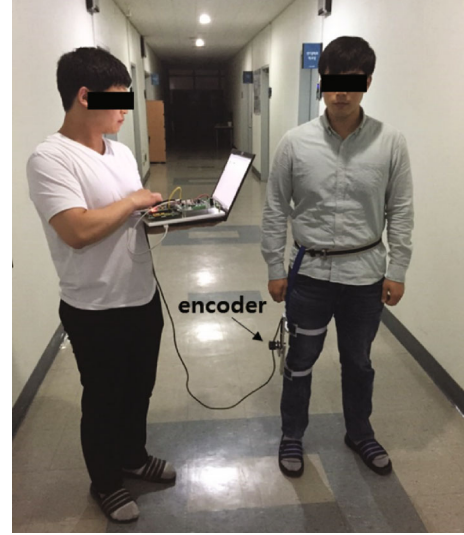
FIGURE 9: Measuring system of the knee motion.
