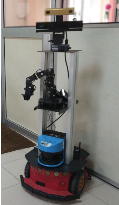
FIGURE 4: Service Robot platform used in the experiment: MIRob.
