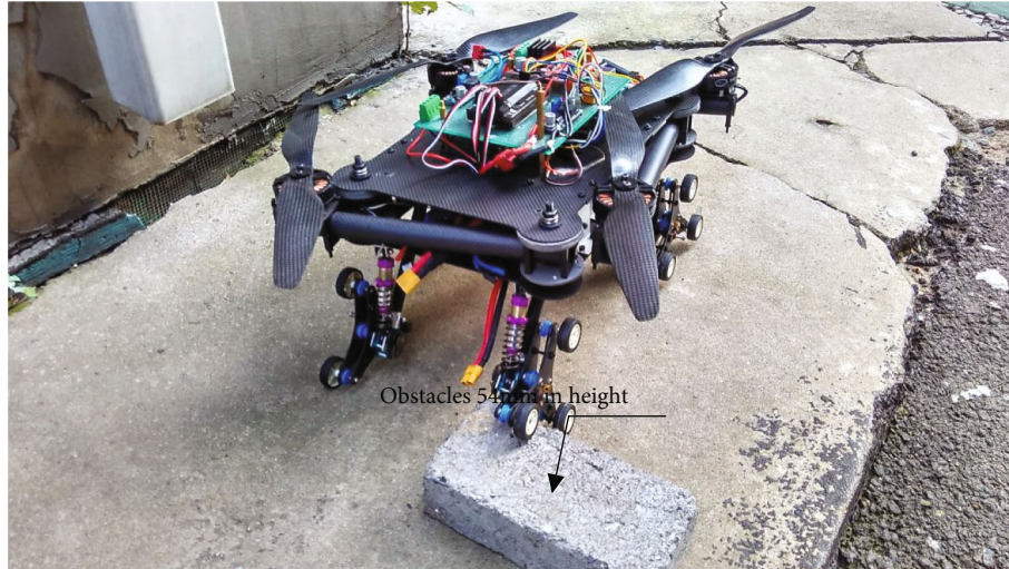
(c) Single planetary wheel climbs obstacle 1
