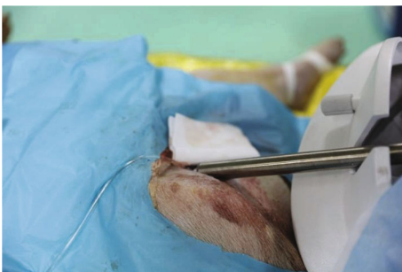
FIGURE 4: The joint between the manipulator arm of the slave end and the femoral artery sheath.
