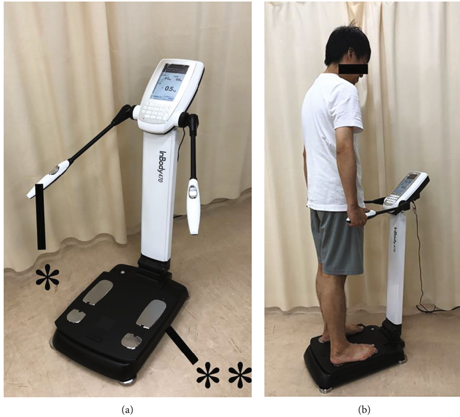
FIGURE 1: Method for measuring body composition. (a) Image of the InBody 470®; *: hand electrodes; **: foot electrodes. (b) Measurement of body composition.
