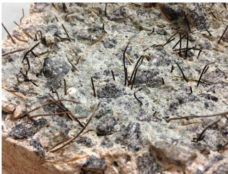
FIGURE 12: Fractured surface of geopolymer concrete showing fibre straining.
