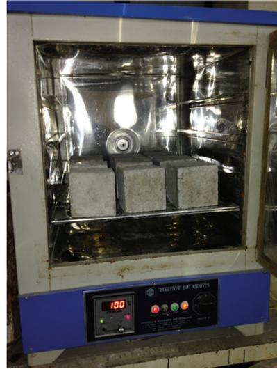
FIGURE 1: Geopolymer concrete specimens cured in hot air oven curing.
