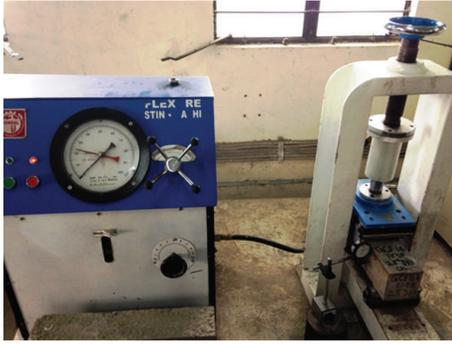
FIGURE 3: Third point loading arrangement in flexural strength testing machine.
