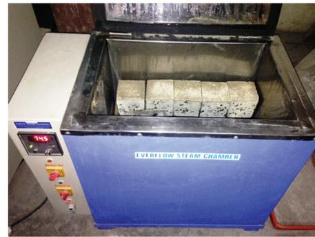
FIGURE 2: Geopolymer concrete specimens cured in steam chamber curing.
