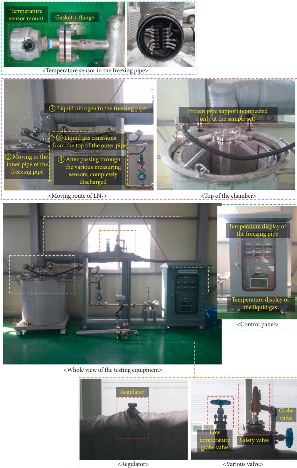
FIGURE 1: Developed ground freezing system.
