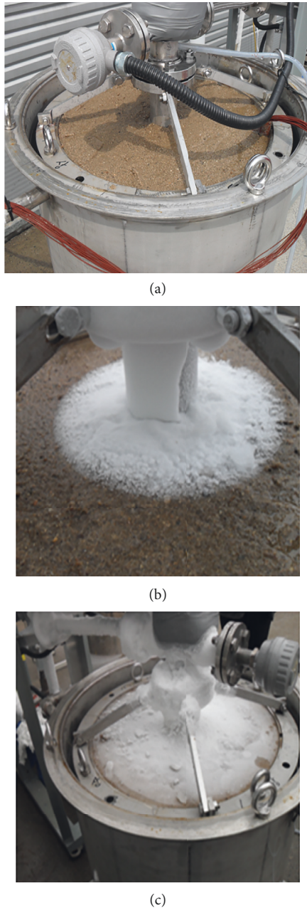
FIGURE 5: Progress of freezing on top of the sand sample.
