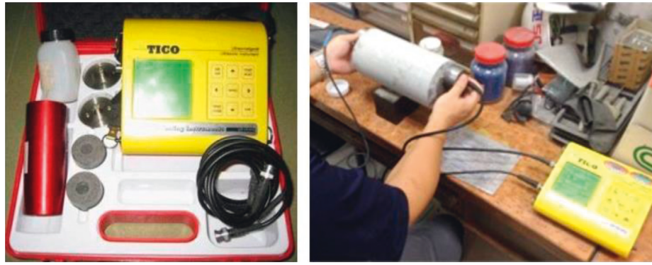
FIGURE 4: Ultrasonic pulse velocity test and TICO ultrasonic pulse velocity.
