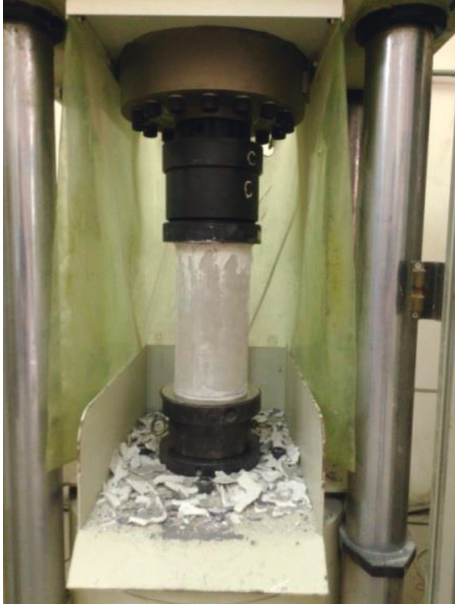
FIGURE 3: Concrete compressive strength test.
