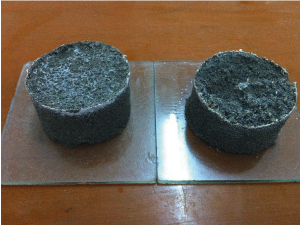
FIGURE 6: Uranium tailings reinforced by MICP.
