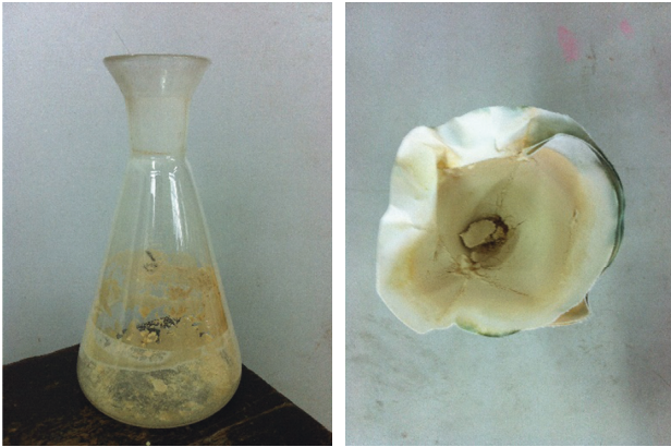
FIGURE 5: The residues in the conical flask and on the filter paper after drying.
