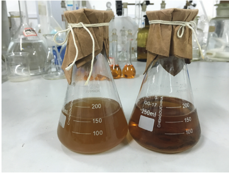
FIGURE 4: Sporosarcina Pasteurii strains were cultured in liquid medium for 2 days (left side is inoculated conical flask and the right side is blank reference).
