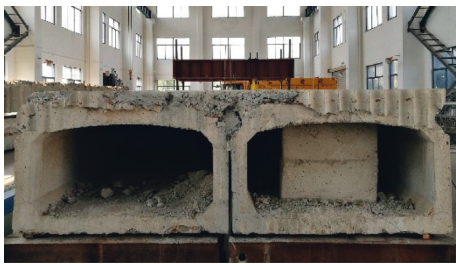
FIGURE 4: Hollow slab prototype test.
