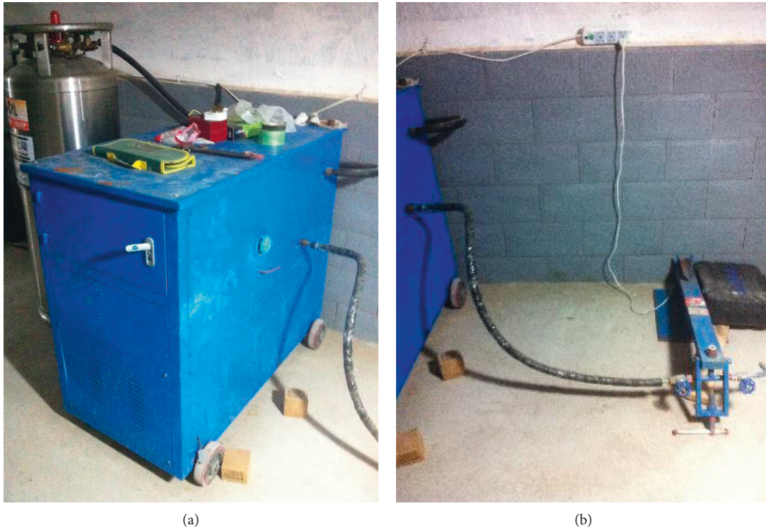
FIGURE 3: Liquid carbon dioxide filling system.
