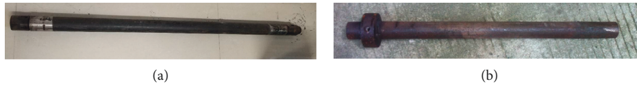
FIGURE 6: Comparative diagram between the conventional fracturing device and the restructured fracturing device. (a) Conventional liquid carbon dioxide fracturing device. (b) Restructured liquid carbon dioxide fracturing device.
