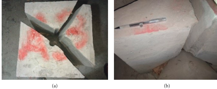
FIGURE 12: The exploded A3 sample after liquid carbon dioxide blasting.
