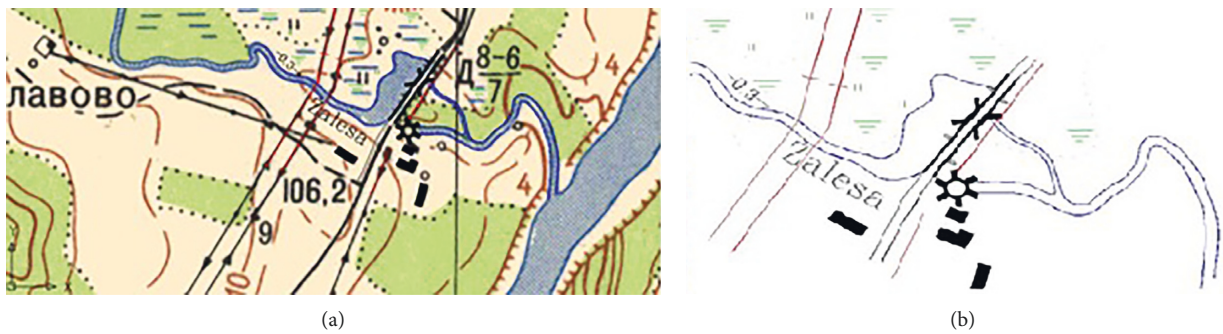
FIGURE 7: Digitized section of River Žalesa is represented in the topographic map of 1972 (source: http://www.geoportal.lt and authors' digitalization).
