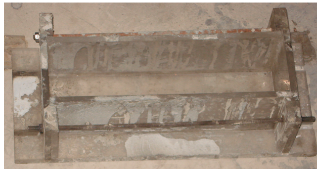
FIGURE 7: The glass mold for measuring free tensile strain.
