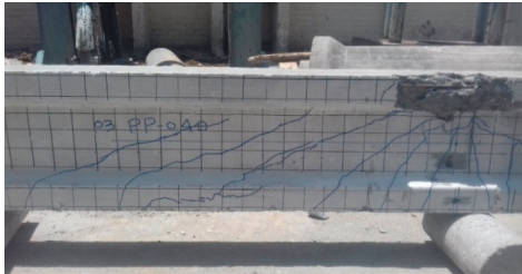
FIGURE 16: Crack patterns of B2-HyFRC.
