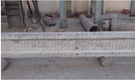
FIGURE 16: Crack patterns of B2-HyFRC.
