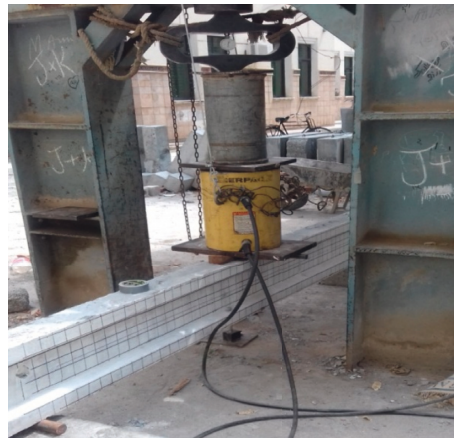
FIGURE 3: Actual test setup using centre point loading.
