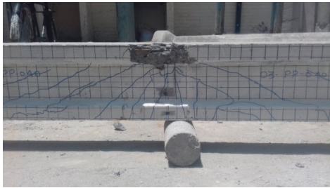
FIGURE 17: Crack patterns of B3-PPFRC-1.
