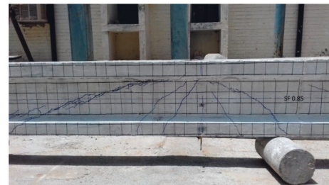
FIGURE 20: Crack patterns of B6-SFRC-2.
