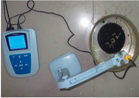
FIGURE 6: Conductivity meter for salt precipitation measurement.
