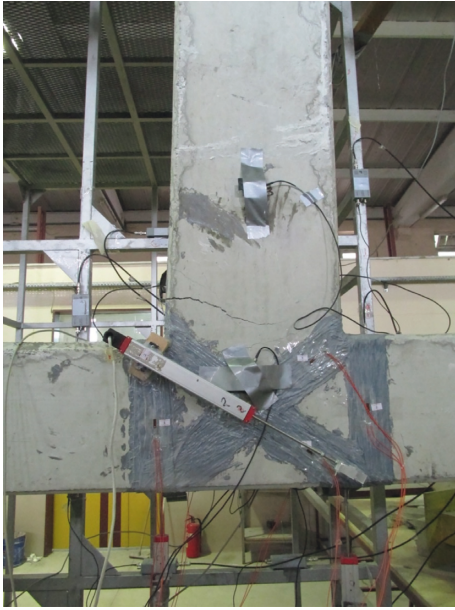
FIGURE 11: Failure of Sample 1.
