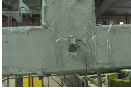
FIGURE 15: Failure of the target sample.
