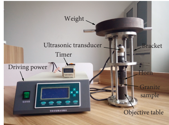
FIGURE 4: Ultrasonic high-frequency excitation experimental device.
