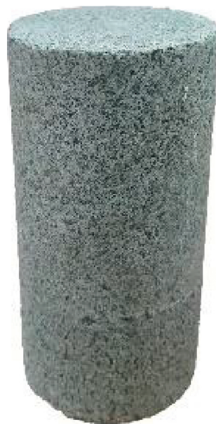
FIGURE 3: Tonalite specimen for uniaxial compression test.
