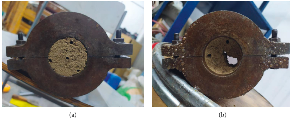
FIGURE 12: One comparison of the initial cracks and destroyed soil layer: (a) initial cracks of experiment No. 21; (b) cracks broaden lead to soil destruction of experiment No. 21.
