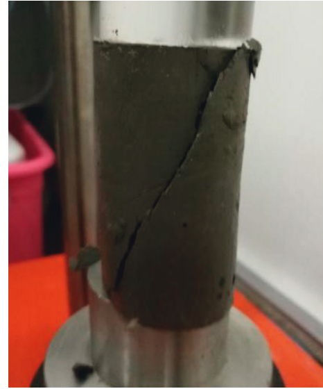
FIGURE 4: Failure mode of cement-admixed slurry specimen with a cement content of 20%.
