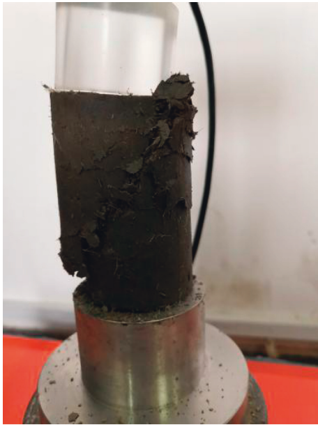
FIGURE 5: Failure mode of cement and fiber admixed slurry specimen with a cement content of 20% and a fiber content of 1%.
