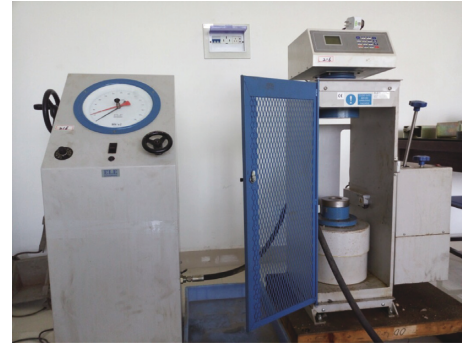
FIGURE 3: Testing equipment for triaxial compression.
